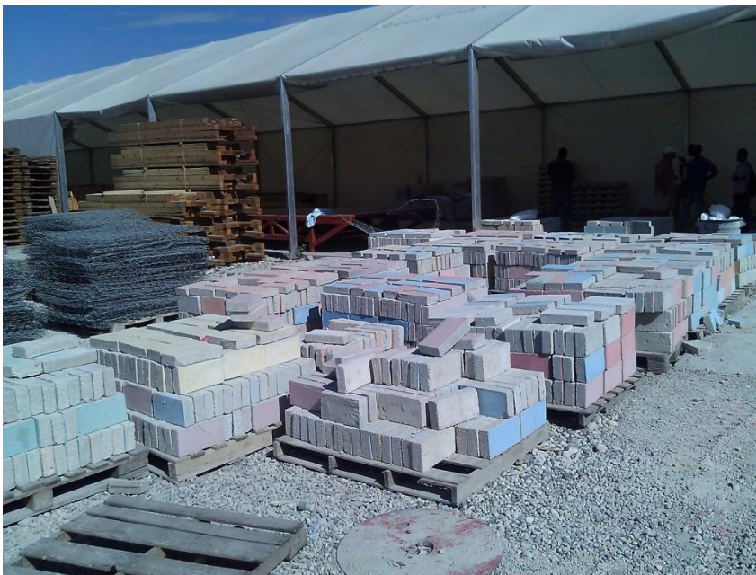
IFRC paving slabs made from reprocessed rubble
