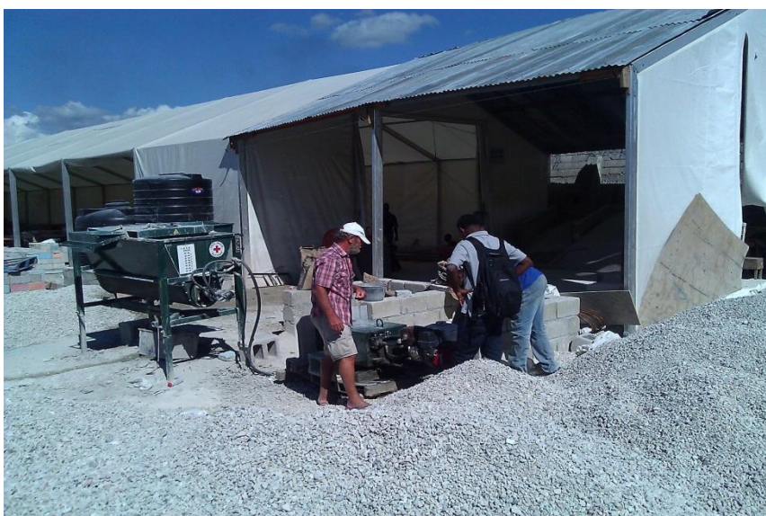
Aggregate produced from earthquake rubble
